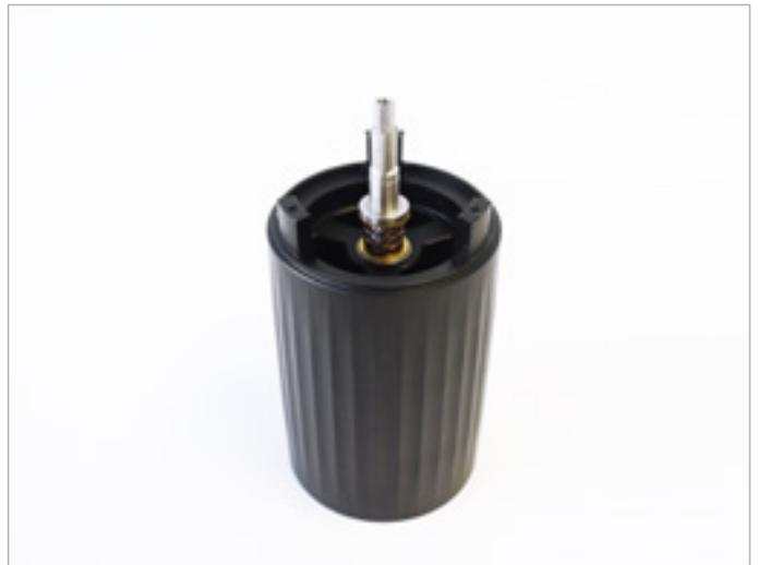
Insert the top of the shaft into the bottom of the upper enclosure and triple spoke plate.
