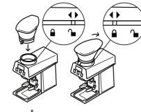
Insert hopper, ensuring that the hopper lock indicator lines up in the unlocked position. Gently turn the hopper clockwise until the hopper lock indicator lines up in the locked nosition.
