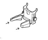
Slide the rubber pads back on to the fork until fully seated.
