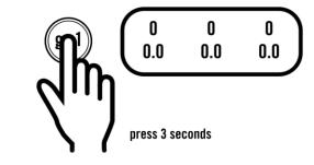
navigate the machine menu by pressing the buttons 1 & 2 to "configure gateway" and press 3 to access it,
