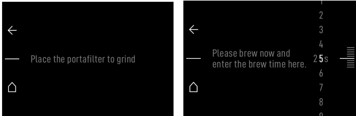
Figure 12; Assisted Dial-In. Refine process and communication of new recipe with the coffee machine.
