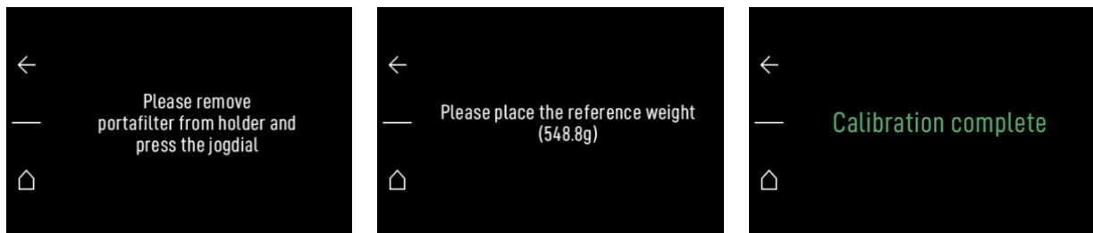
Figure 25; Load Cell calibration process
