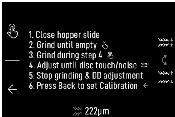
Figure 26; Disc Distance Calibration Process
